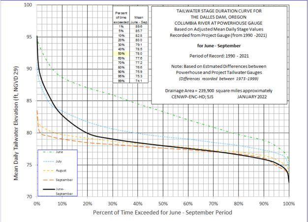
Figure 3-6. The Dalles Tailwater Elevation versus Percent of Time Exceeded for June - September.
