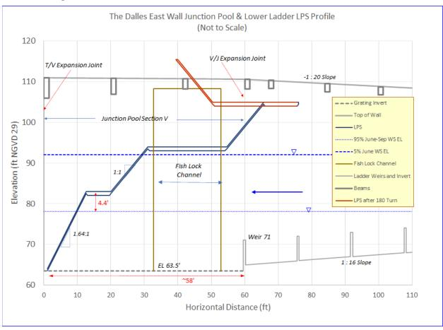
Figure 3-16. The Dalles East Wall Junction Pool & Lower Ladder LPS Profile
