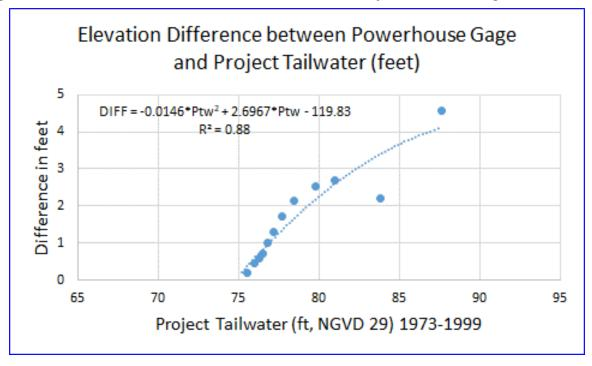
Figure 3-5. Elevation Difference between Powerhouse and Project Tailwater Gauges.
