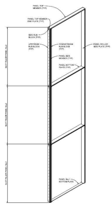
Figure 4-1. Frame style slot filler to be used for this project
