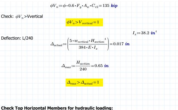
HSS 8x2x5/16 in strong axis direction. The only difference between this and vertical members is the span distance. Both are loaded in the strong axis orientation
