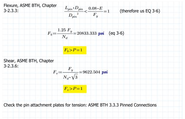
BTH, slenderness, tensile strength through a pinhole (3-45), single plane fracture strength beyond the pin hole (3-49) 3-3.3.1, double plane shear strength beyond the pinhole (3-50), bearing stress (3-53).
