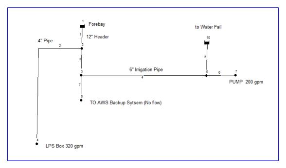
Figure 3-12. Plan EPANet Schematic of LPS and Irrigation Supply Pipe Systems
