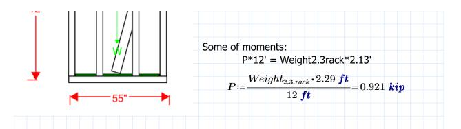
It is reasonable to assume a 2k lb slot filler cannot produce a .921 kip force at the top of the storage rack by leaning. Therefore, the rack is stable. However, the more wide the more stable.
