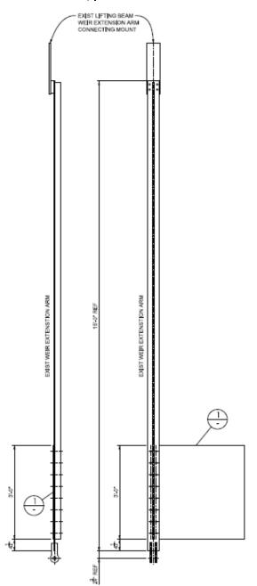
Figure 4-3. The Dalles Dam, plate slot cover attached to lifting beam
