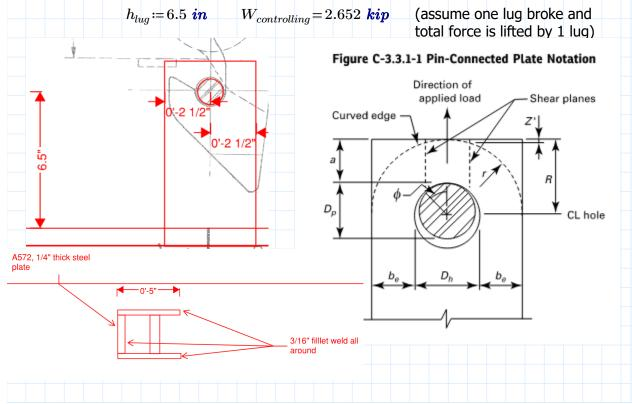
Static strength of the plates: ASME BTH EQ, 3-45
