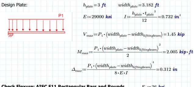
Check Flexure: AISC F11 Rectangular Bars and Rounds $F_y := 36 \ ksi$ Yielding: $Z_x := \frac{h_{plate} \cdot t_{plate}^2}{4} = 3.516 \ in^3$  $S_x := \frac{h_{plate} \cdot t_{plate}^2}{6} = 2.344 \ in^3$
