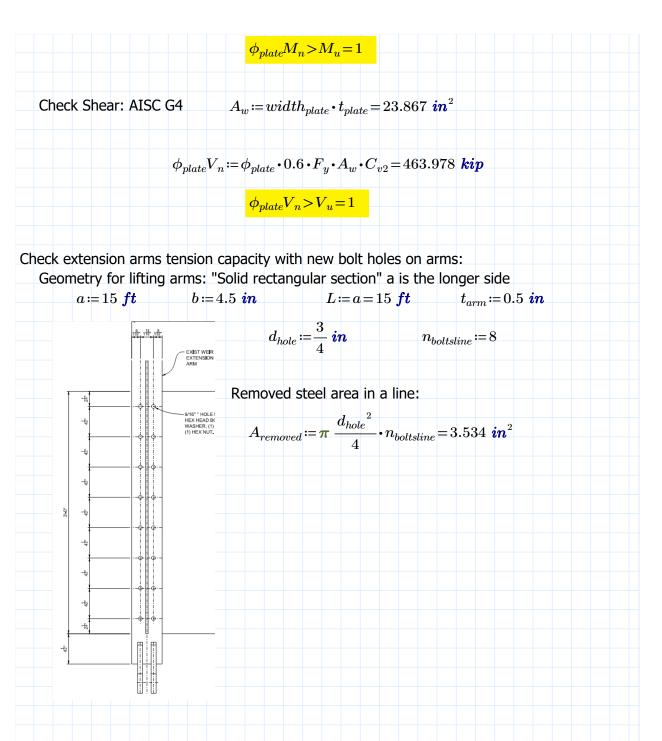
Check Lifting Arms for Torsion, AISC H3 "Non-HSS Members subject to torsion and combined stress: OR use roark stress and strain pg. 389
