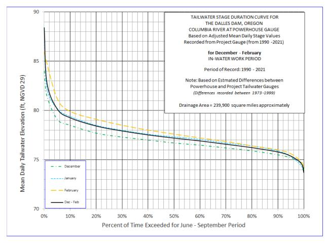
Figure 3-7. The Dalles Tailwater Elevation versus Percent of Time Exceeded for In-Water Work Period.
