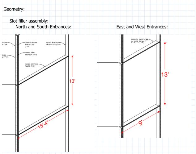
Design the larger rack and size the smaller one based on those calcs. The bigger rack will control due to high loads.
