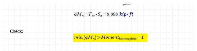
Check with penetration: AISC F13, Strength reductions for members with holes in tension flange
