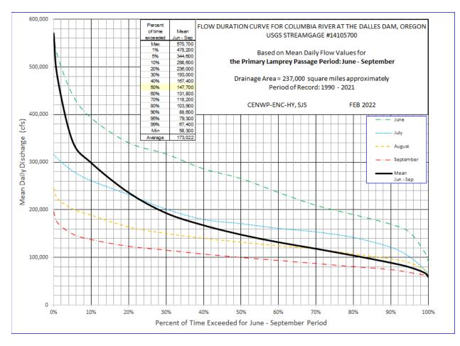
Figure 3-2. The Dalles Project Discharge versus Percent of Time Exceeded for the June -September
