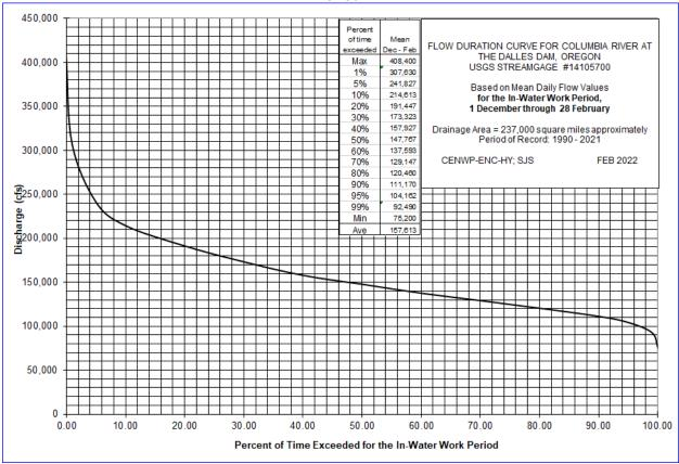
Figure 3-4. The Dalles Project Discharge versus Percent of Time Exceeded for the In-Water Work Period.
